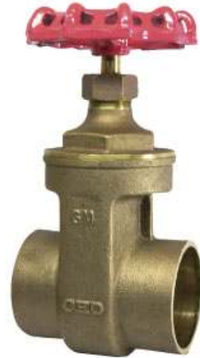
Model 102C Pneumatic pressure test: 6 Kg/cm 2 (Air Under Water) 200 psi W.O.G. Non-shock
